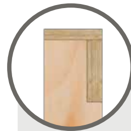
Notched stud with continuous lintel
