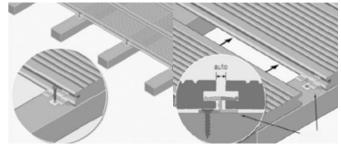
1 Clip per joist has to be placed to the grooved sides of the board. Do not use one Clip to fasten two boards together where two boards meet end-to-end over a joist. To add additonal blocking, we recommend adding a 20 cm block and using a clip (at least 15 cm from the end of board) at the end of each board (see Figure 2).
