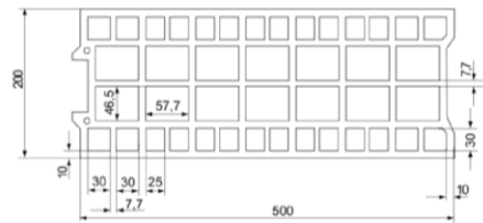
Vertical perforated brick HLz, form B, EN 771-1 Producer e.g. Bouyer Leroux Nominal dimensions [mm] length L width W height H 500 200 315 Density \rho [kg/dm 3 ] ≥ 0,6 Compressive strength f_b [N/mm 2 ] 4 / 6 / 8 Standard or annex EN 771-1
