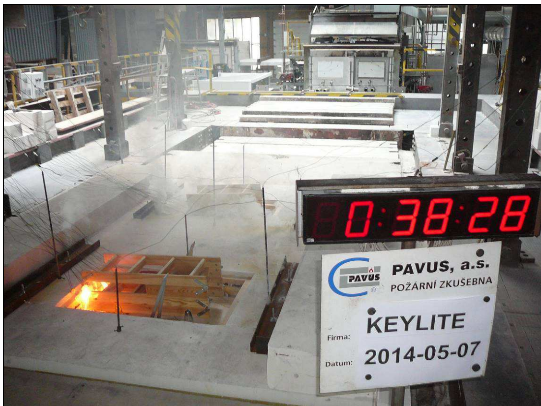
End of test, integrity failure of specimen No. 2 – 39 th test minute
