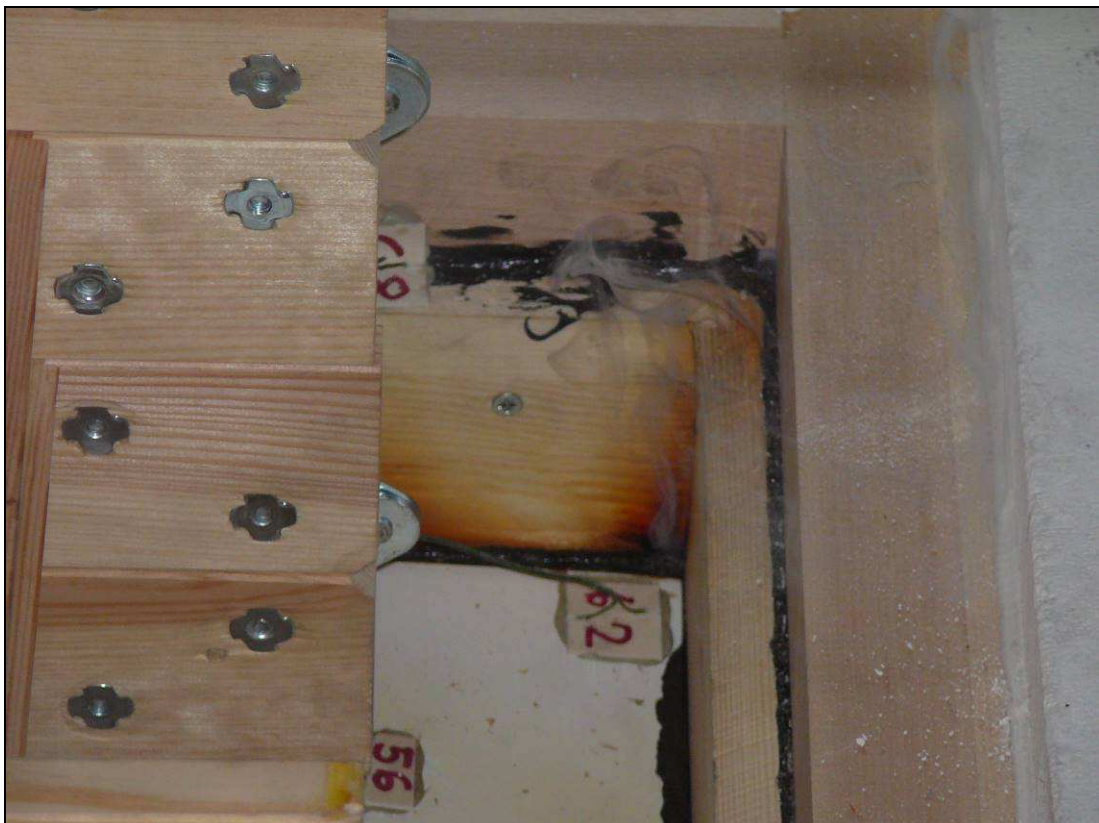
Specimen No. 2 – reaction of intumescent tape in gap – 20 th test minute
