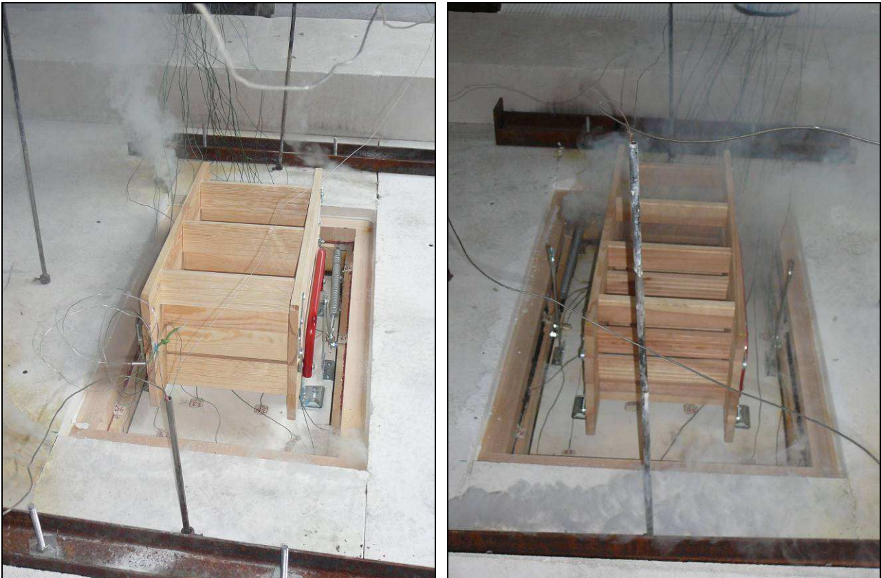
Specimen No. 1 and 2 – 31 st test minute
